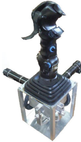
Figure 8. (Colour online) The assembled force-feedback side-stick.
